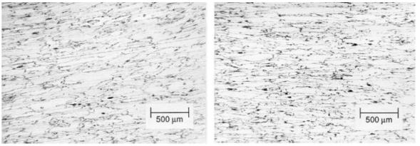
Fig. 6a and 6b: Homogeneous distribution of antistatic modifier
