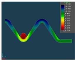
Fig. 4b: FEM Calculation of tangential stress
