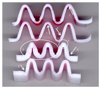
Fig. 2: Unacceptable defects that reduce the performance of the PTFE bellow
