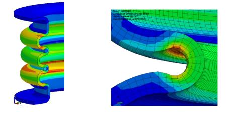
Fig. 9a and b: Simulation of the maximal operation pressure before plastic deformation; Source SGL / Dr. Schnabel GmbH
