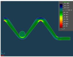
Fig. 4a: FEM Calculation of axial stress
