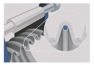
Fig. 13: Vacuum rings to increase the vacuum resistance; Source SGL / Dr. Schnabel GmbH
