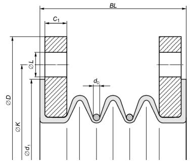
Fig. 11: Design of a PTFE-axial expansion joint; example for a three comvolution layout
