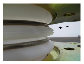
Fig. 5: Crack initiation after <5000 axial movement cycles due to an inhomogeneous distribution of the wall thickness
