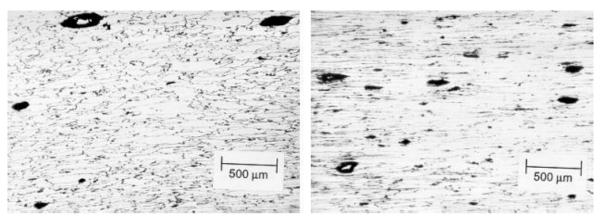
Fig. 7a and 7b: Inhomogeneous distribution, does not comply with the requirements
