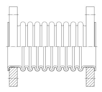
Fig. 12: High pressure expansion joint with internal PTFE liner
