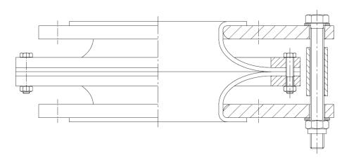
Fig. 14: POLYFLURON<sup>®</sup> vacuum expansion joint FX-0; source SGL / Dr. Schnabel GmbH
